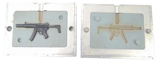
The tested polymers are listed in the table below and include PP, PE, HDPE, ABS, PETG, PA6 and PA12 co-polymer, injected at temperatures between 230 and 280°C (446 - 536°F). All materials were injected without any mold release agents.
